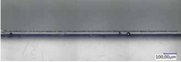
Blade cut of plastic film
