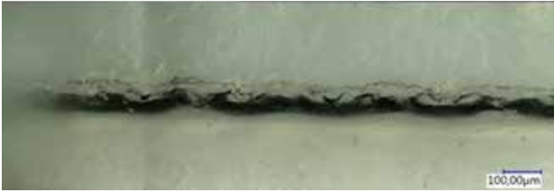
Blade cut of plastic film
